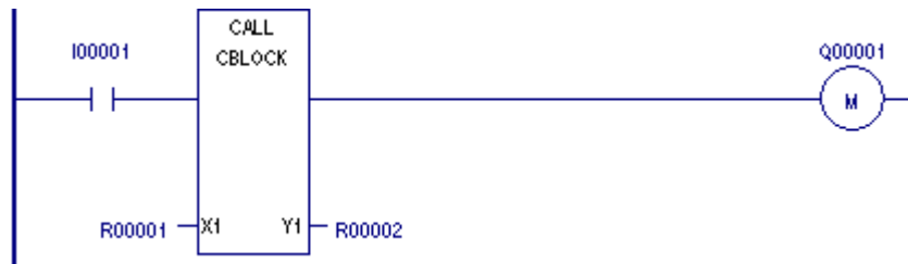
Figure 3-2. Invoking a C block from Ladder Program
